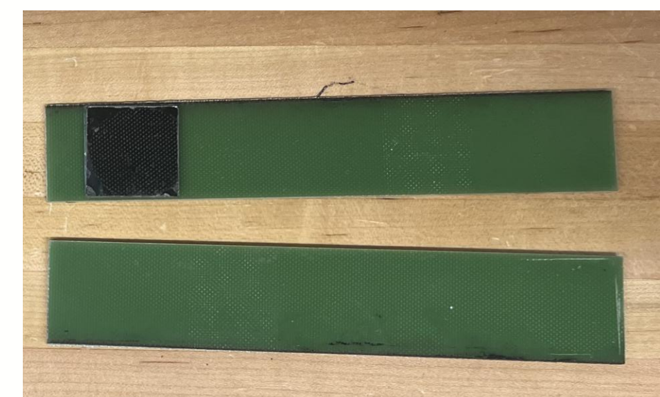
Sample 1: Adhesion failure at glass/epoxy interface (higher surface roughness)
