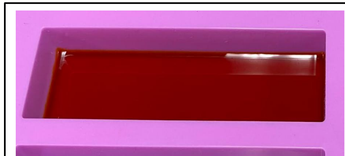
Figure 1. Image of synthesized polyurethane film loaded with Rifampicin.
