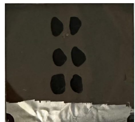
Figure 4 (a) Carbon shows minimal to no degradation
