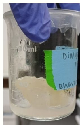
Fig. 5. Gel substance formed during dialysis with stored LiBr.
