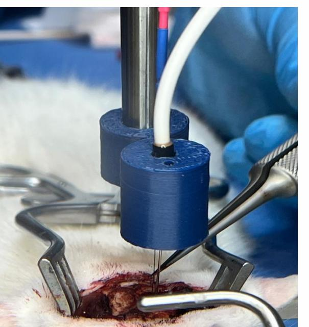
Fig 4: Working electrode along with reference electrode employed in-vivo at the craniotomy site.
