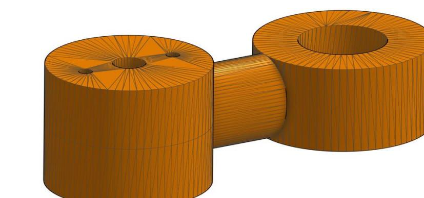
Figure 3: CAD model of the apparatus used to hold the 3-electrode system.
