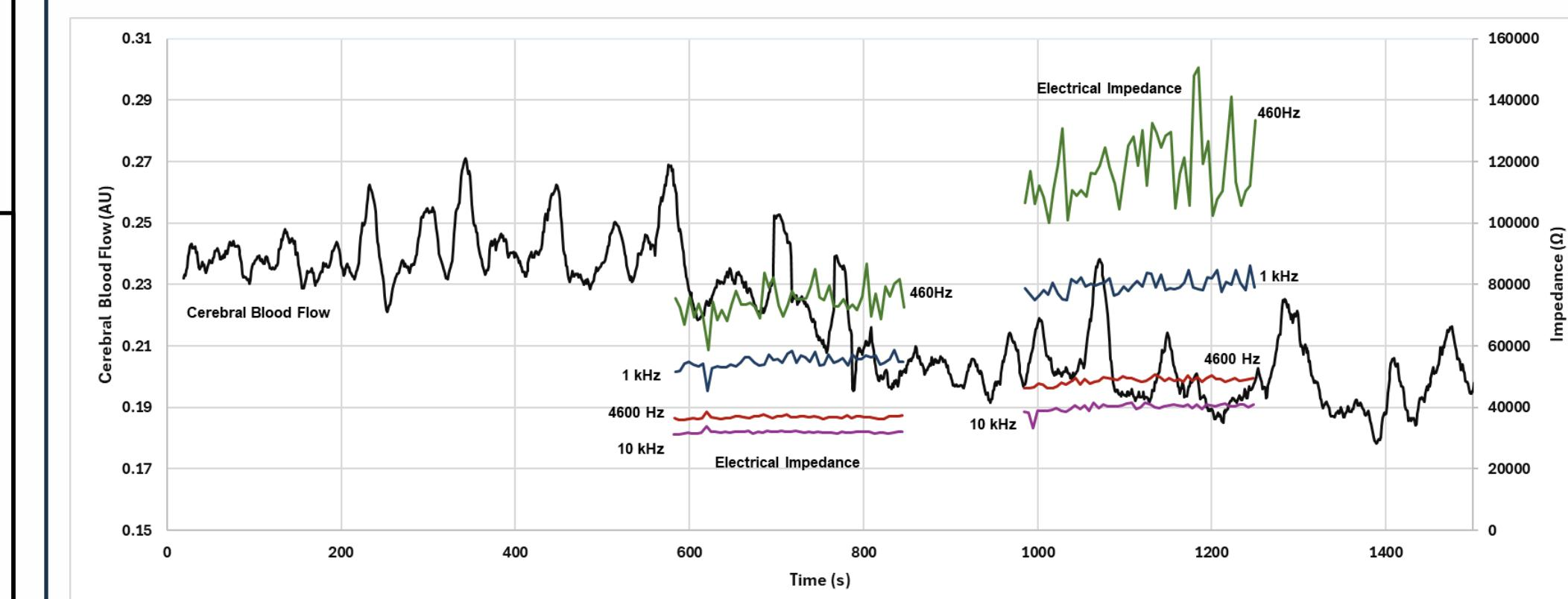
Fig.8. Plot showing changes in both local cerebral blood flow from the laser doppler flow probe and electrical impedance of brain tissue at 460 Hz, 1 kHz, 4600 Hz and 10 kHz plotted as a function of time. Increase in electrical impedance coincides with decreasing blood flow.
