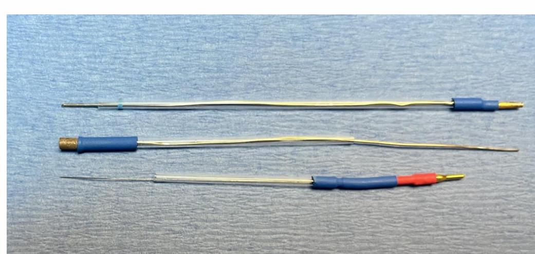
Figure 2 : Tungsten (red), Platinum-Iridium and Ag/AgCl electrodes used for EIS measurements.
