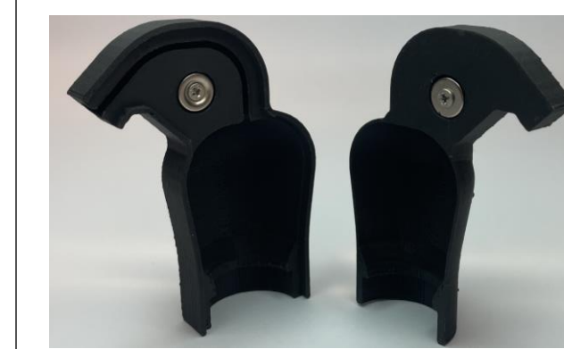
Figure 8. Final optical fiber loading instrument. Fiber is loaded through opening on left partition and tip is secured with a bare fiber optic terminator clip (Thorlabs, BFT1). Ambient light is blocked by attaching the two partitions using magnets around the fiber. The other tip of the fiber is loaded into the patch-clamp electrophysiology system.
