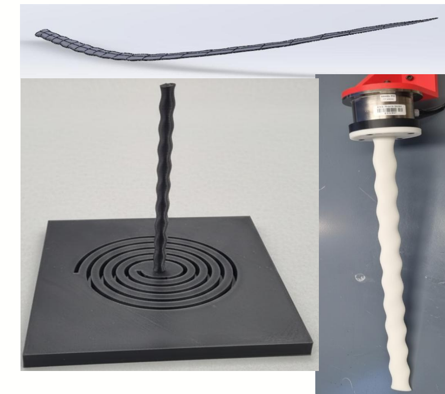
Fig 2: 3D CAD Model and Printed Whisker Prototype
