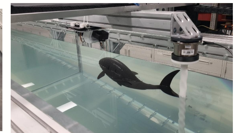
Fig 7b: Test Configuration: Seal Whisker with Robotic Fish developed for this study
