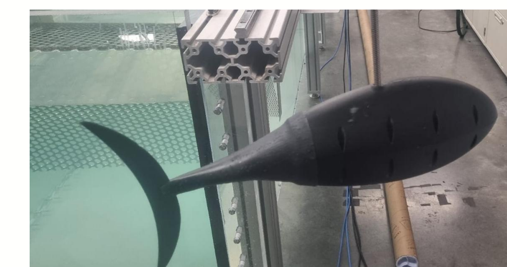
Fig 7a: Bio-mimicked Robotic fish developed for this study
