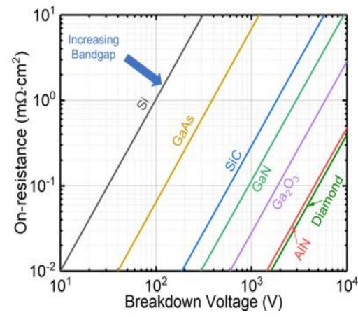
UWBG devices have greater performance than WBG devices with their larger band-gap leading to higher breakdown voltage, higher critical electric field and larger Baliga's figure of merits
