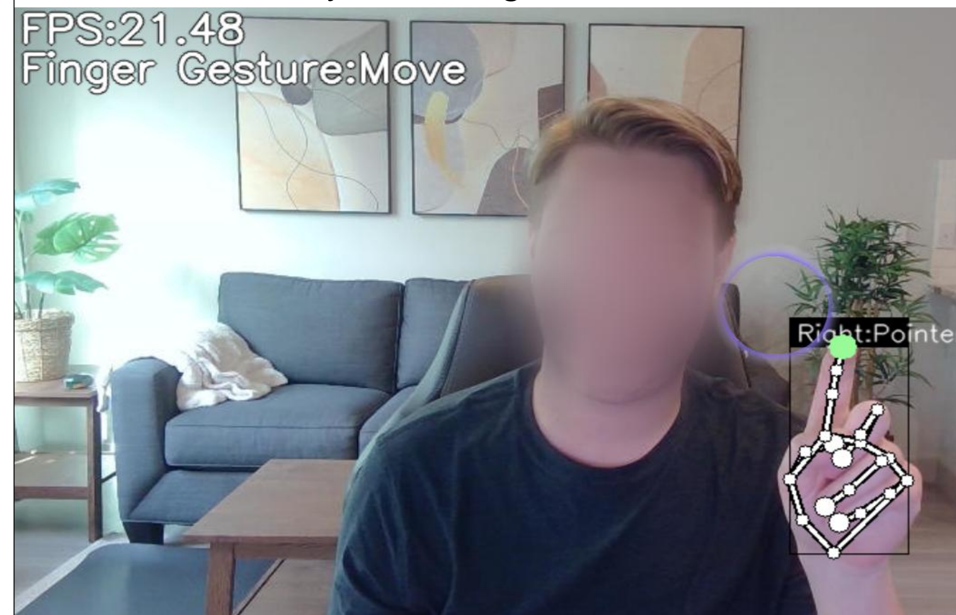
Figure 1: Software's View for Hand Gesture Recognition and Eye Tracking (The Blue Circle is the Gaze Location)
