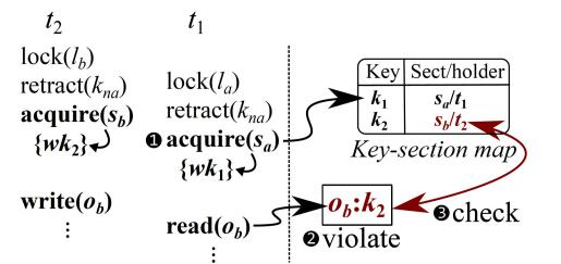
c. Conflicting access across threads raises a fault, which is checked for race conditions.
