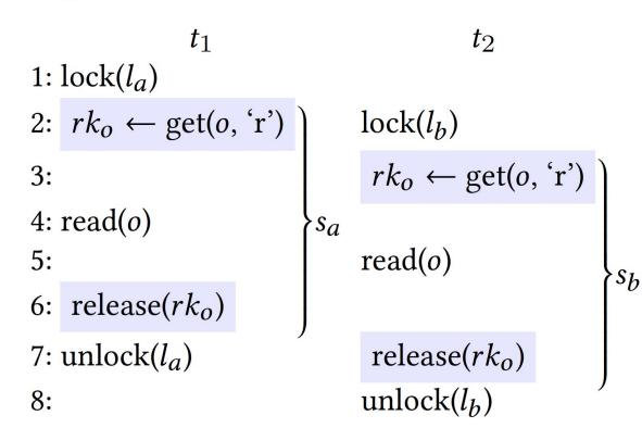
(b) Shared read.  $t_2$  can obtain  $rk_o$  to read from o while  $t_1$  is holding  $rk_o$ .
