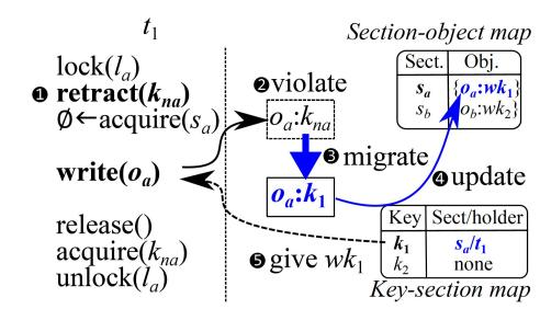
a. First access triggers a fault and object migration into a protected domain.
