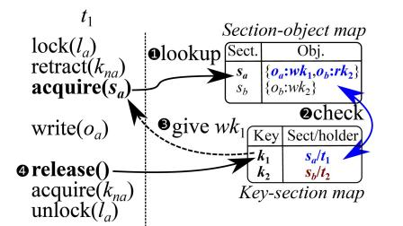
b. Protection keys are granted upon critical section entry based on tracked object.
