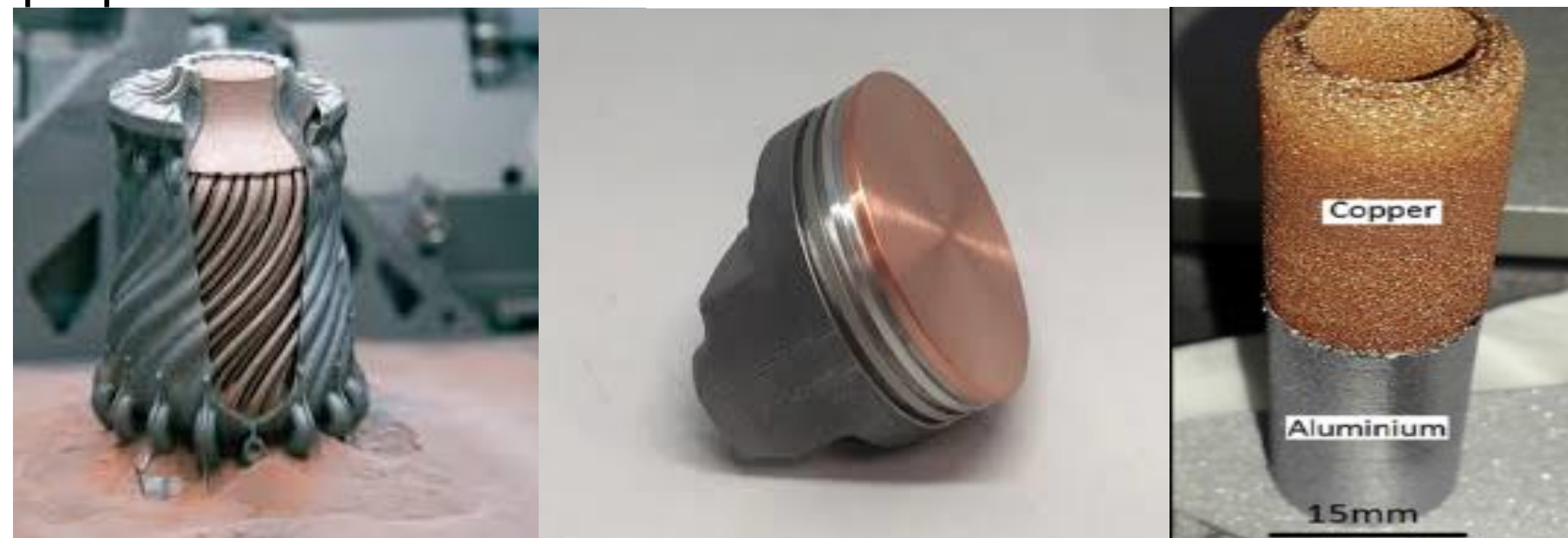
All are examples of multi-metal prints however the right image was created with PBF and is shown to have a poor surface roughness.
