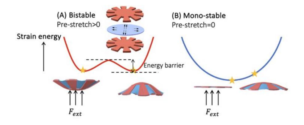
How it works: A pre-stretched elastic membrane with 2 solid structures attached on the top and bottom cause the device to have 2 static positions. Wave motion causes the change between static states. The device harvests electricity from the change in static shapes.
