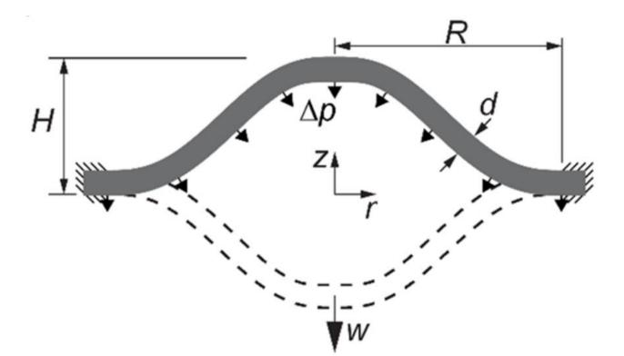
How it works: Monostable viscoelastic materials have a static position and second temporary static position. Using a makeshift vacuum chamber, we can create pressure differences causing the material to enter to temporary static position. Studying its deformation over time can give us insights to the best geometric configurations.
