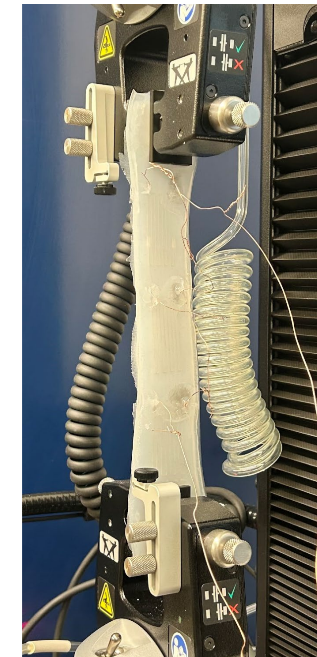
Fig 6: Silicon sensor tested on Instron machine (Left)
