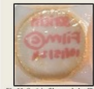
Fig. 11. Sericin film made by film casting
