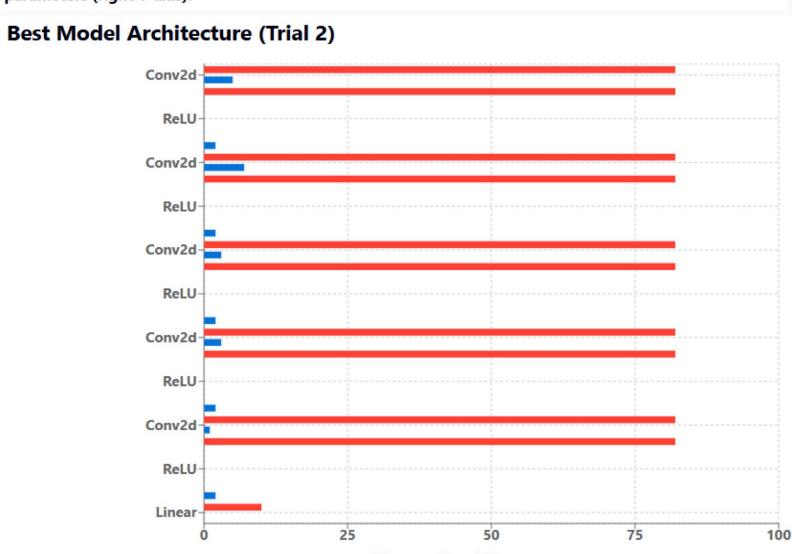
Legend: This chart shows the architecture of the best-performing model from Trial 2. Each row represents a layer in the model. The red bars show the number of filters in each layer, while the blue bars represent the kernel size (where applicable).
