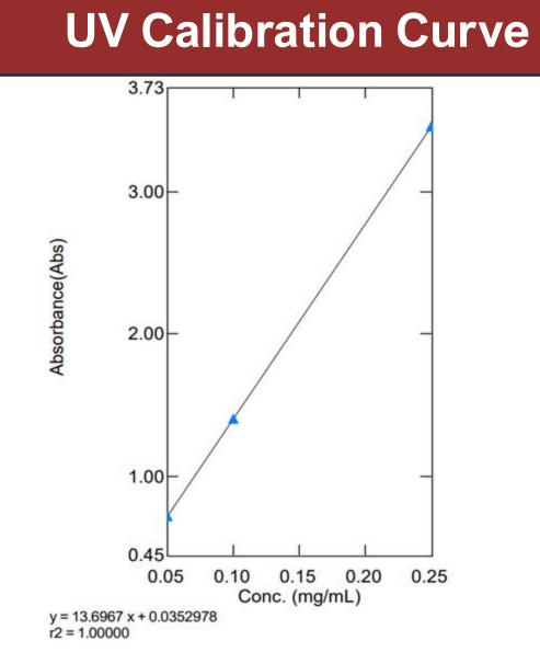
Curve tested at 0.175 mg/ml SnO2: Predicted Concentration: 0.179 mg/ml **Predicted absorbance: 2.483**
