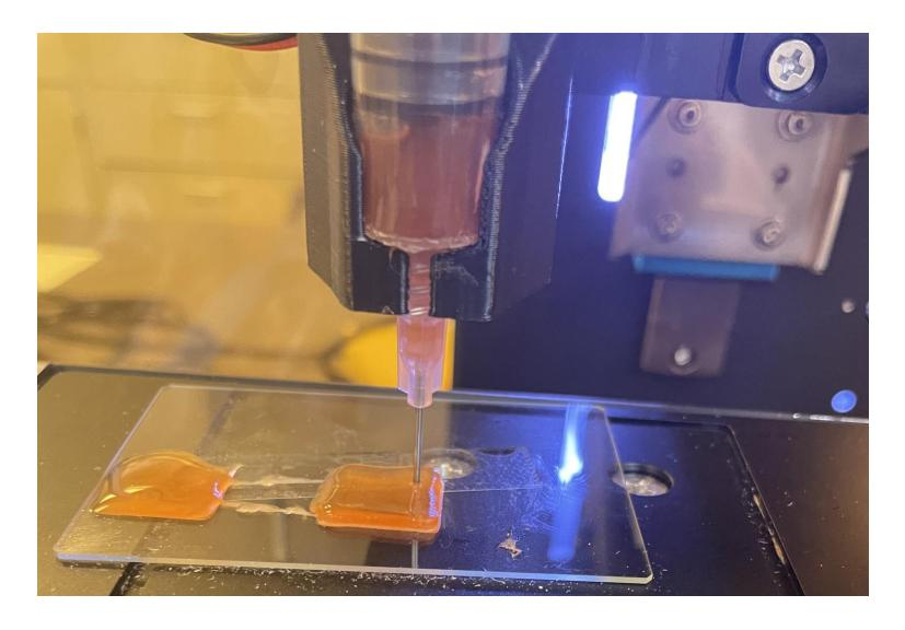
Viscosity and homogeneity vary with time Resin cures and solidifies at the needle tip Each needle tip requires specific flow rate Low viscosity make overhangs challenging
