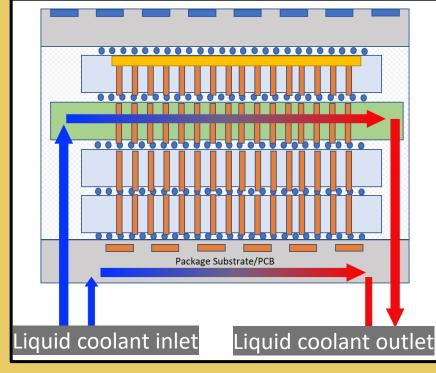
A new class of thermal management system needs to be explored for 3D Packaging and intralayer microfluid cooling is a promising solution.
