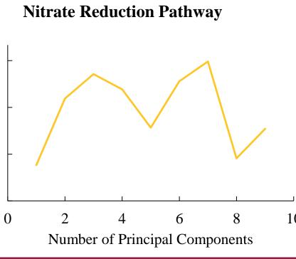
Figure 5. Standard deviation of error (eV) for the *ExtraTrees Regressor as a function of the number* principal components and the best number of estimators for 6 of the reaction steps in the nitrate reduction reaction pathway.
