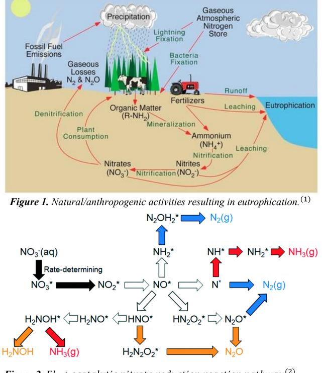
*Figure 2.* Electrocatalytic nitrate reduction reaction pathway<sup>(2)</sup> the economic viability of the electrochemical conversion of nitrate to valuable NH<sub>3</sub> or benign N<sub>2</sub>.
