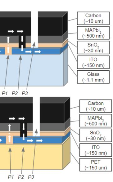
Figure 1. Depiction shows the contents of the MAPI Perovskite Solar Cell that was created for both Rigid (Glass) and Flexible (PET) substrates. Labels for each scribe and
