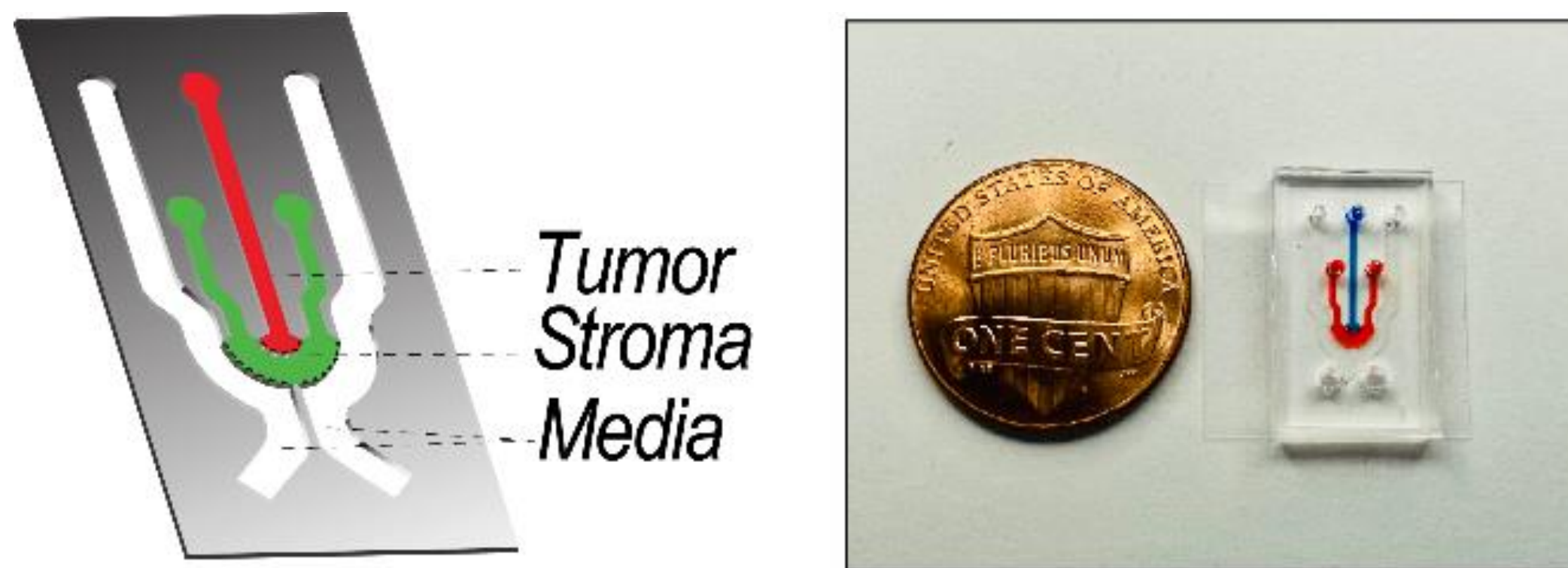
Figure 1: Tumor-on-chip model. Schematic representation of COC microfluidic model with interconnected tumor and stromal region (Left). Actual microfluidic device next to a coin to depict the size of the device (Right).
