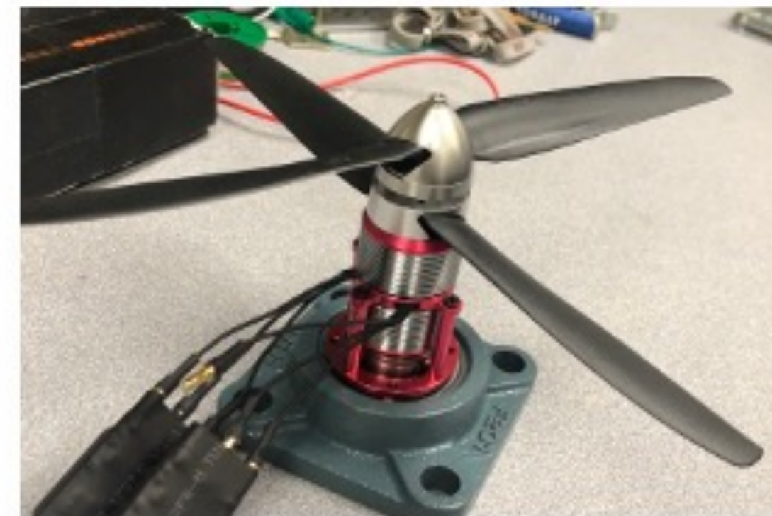
Figure 3: Brushless motors on a base, working with controllers connected with teensy processor (top left)
