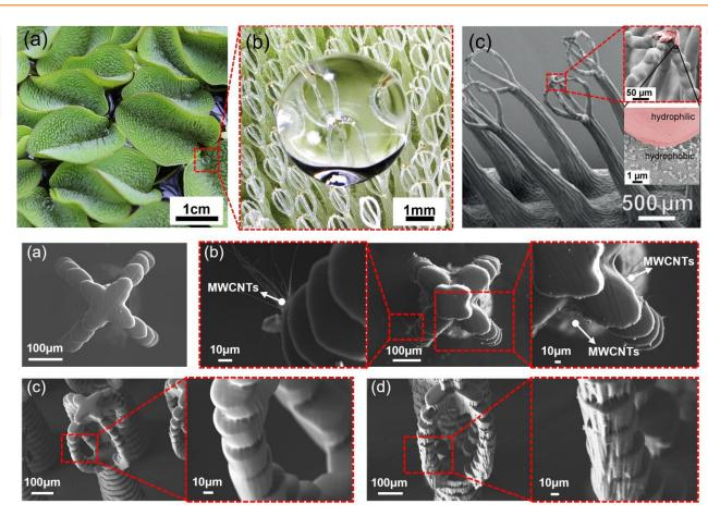
superhydrophobic properties because of its unique eggbeater structures characterized by dual-scale roughness featuring microscale trichomes and nanoscale wax crystals, facilitating stable air retention underwater.
