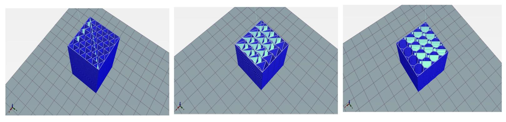
Due to 3D Printing difficulties using TPU and time constraints, only the Re-entrant and Grid pattern were printed and tested. Samples were compressed using a Universal Testing Machine to obtain Stress-Strain Diagrams and were manually compressed and measured for their Poisson's ratio
