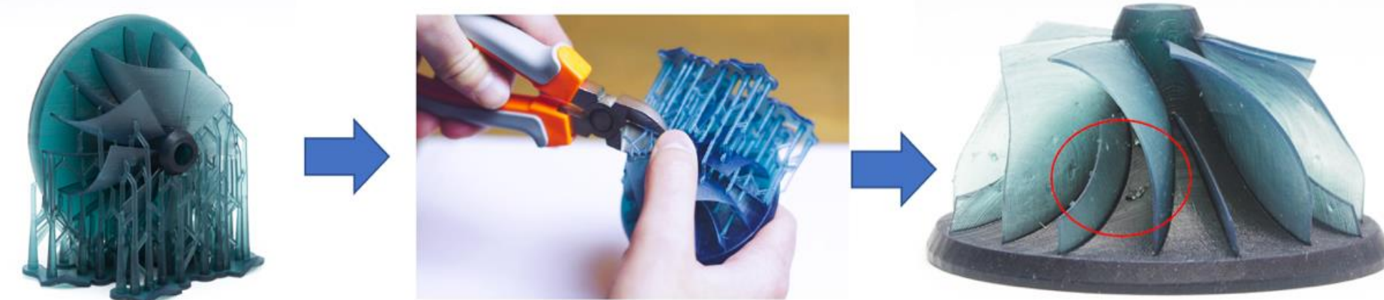
VPP printed object with supports Removal of supports Surface marks
