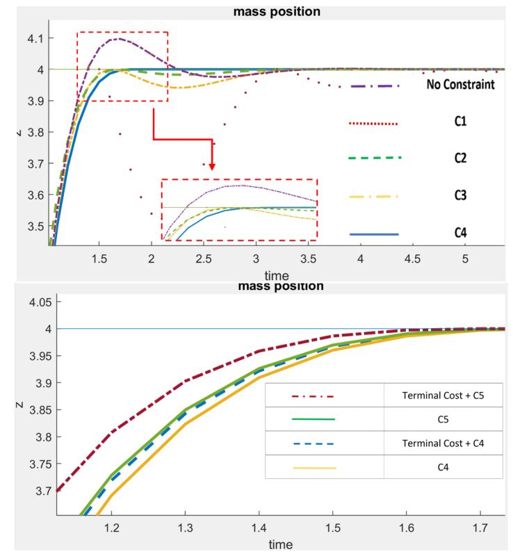
Fig 5 System response for non-linear MPC with non overshooting constraints. terminal cost & C5 From the simulation above we could infer the following characteristics, **Convergence:** *Terminal cost* + *C*5 > *C*5 > *C*4 > C3 > C2 > C1
