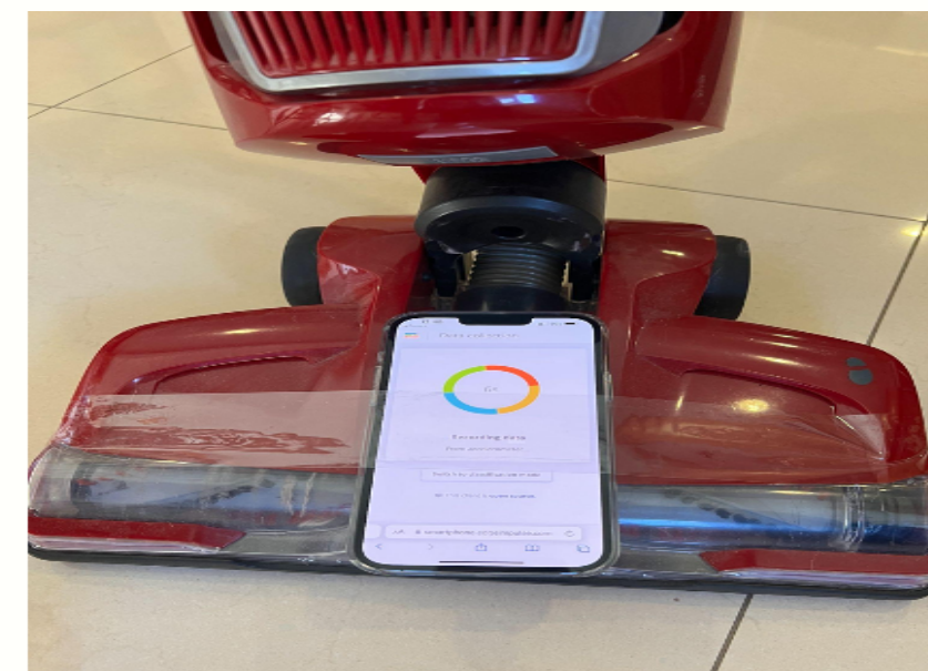
Figure 2: Smartphone attached to Vacuum cleaner for data acquisition
