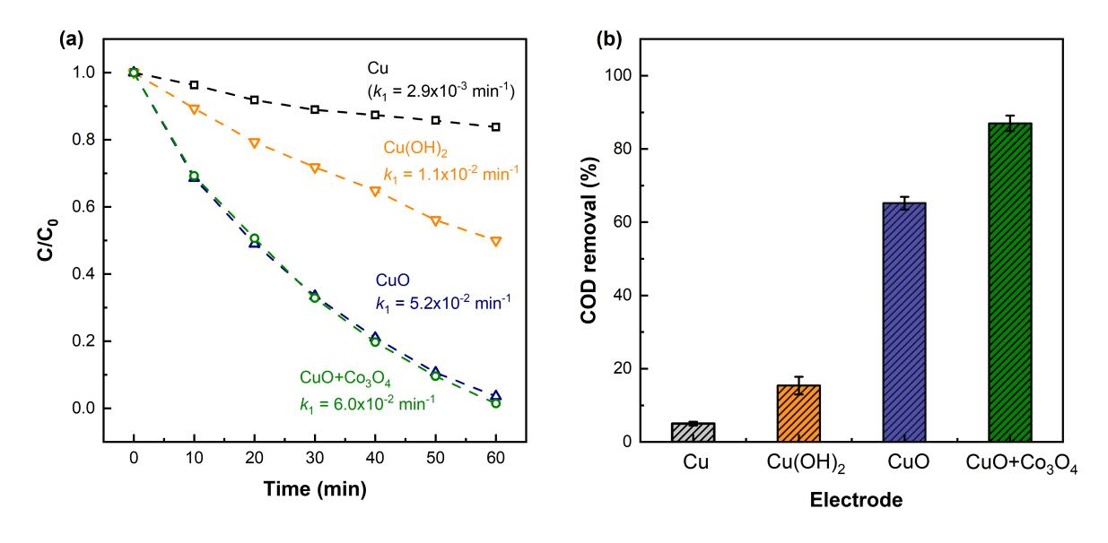
Different electrode configuration was evaluated obtaining (a) different kinetics and (b) COD removal.
