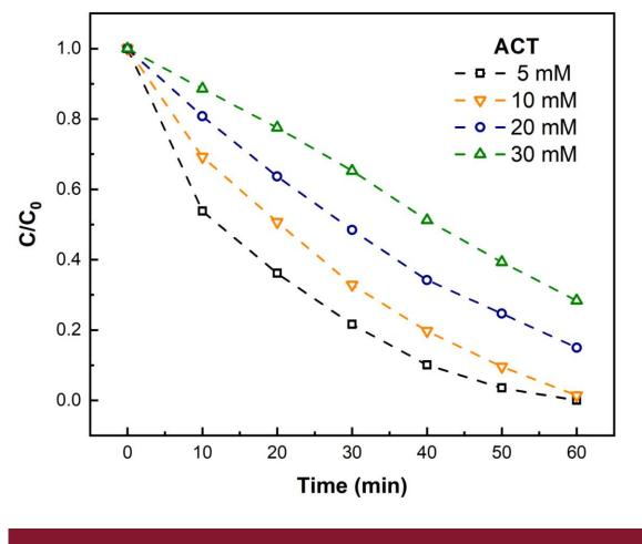
Optimal conditions:  $CuO + Co_3O_4$  4 mM PS $2.0 \text{ mA cm}^{-2}$
