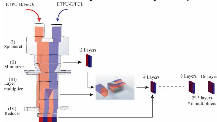
The two feedstock composites are A. TPU 1254D13U / PCL which primarily features high-temperature sensitivity and B. TPU B60A 10 WHTSG000 / Fe<sub>3</sub>O<sub>4</sub> which primarily features high strength and magnetic stability. The resulting composite is intended to exhibit a compromise of both feedstock characteristics and produce both thermal and magnetically controlled actuation.
