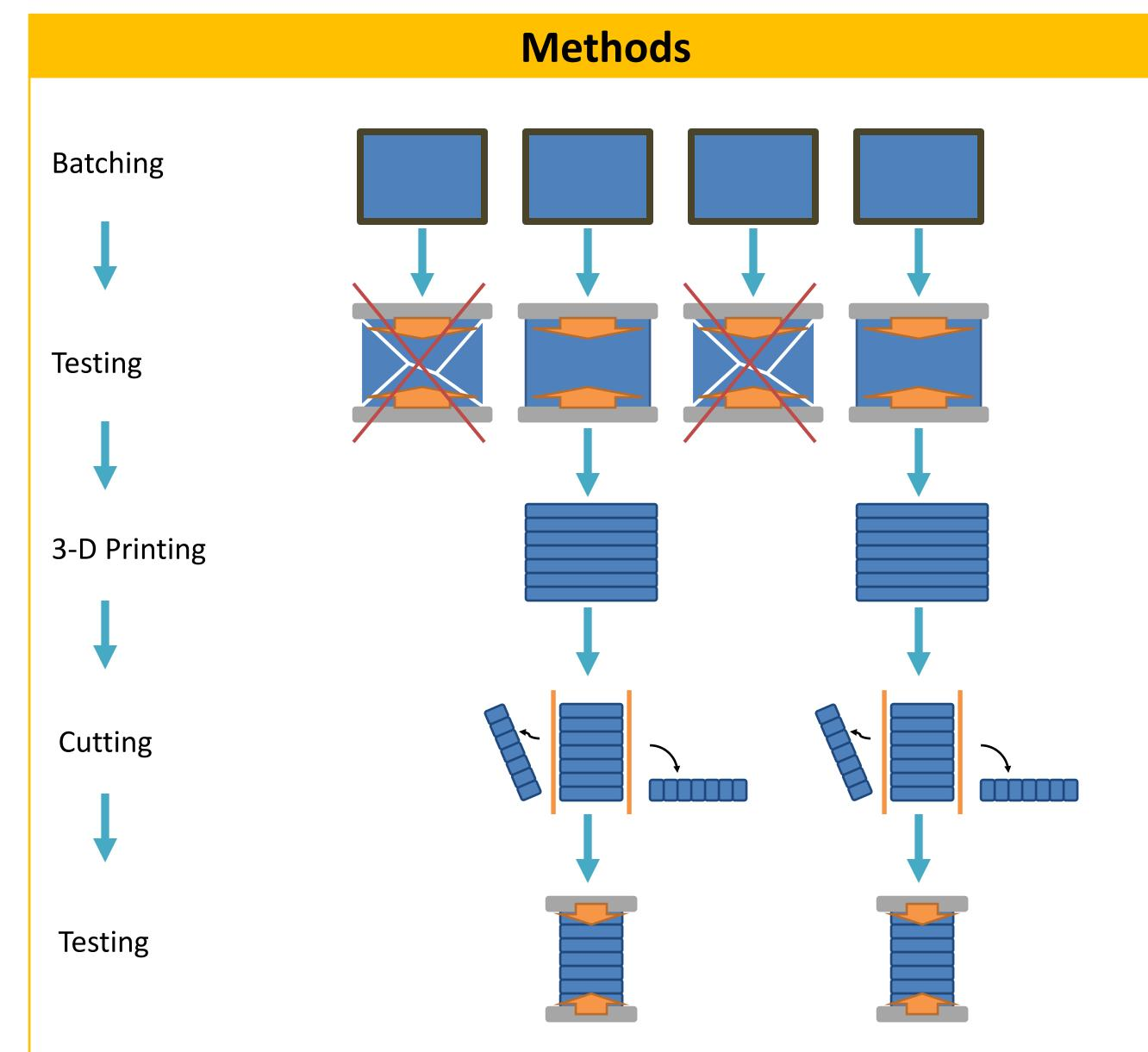
Batching: Multiple concrete mixtures are cast into approximately 2-inch cubes.
