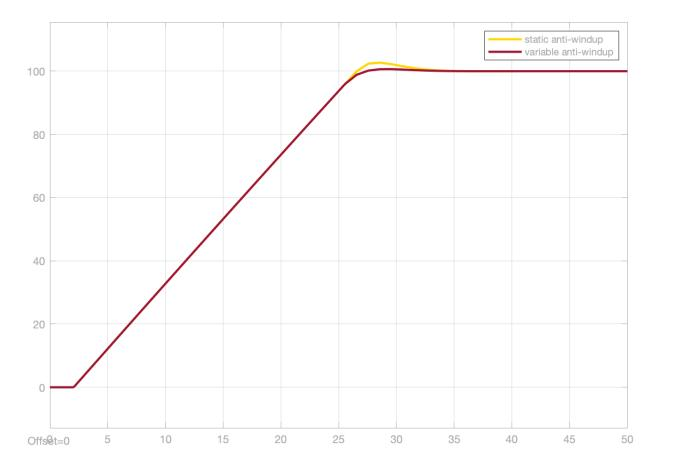
Controlled  $\dot{z}$  with static and variable anti-windup
