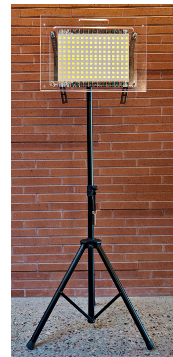
Final design of the THz lab reflectarray with the completed bias PCB on the back
