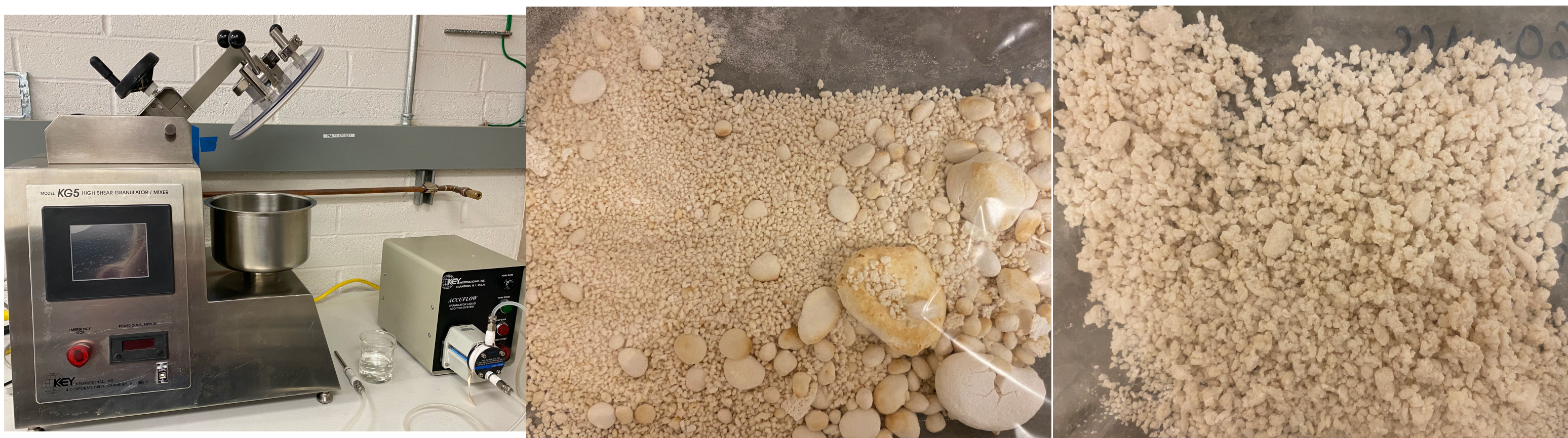
Figure 2: Experimental Setup Figure 3: 100% MCC Resulting Granules Figure 4: 60% MCC Resulting Granules
