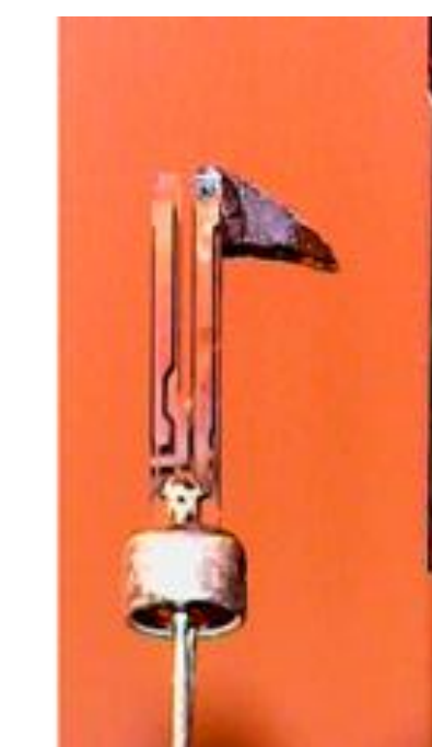
Akiyama Probe fixed on a tuning fork (L) under a microscope and a silicone tip probe on a tuning fork (R).
