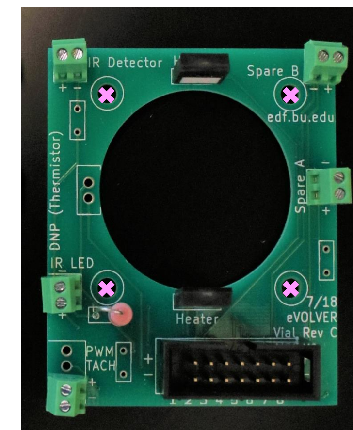
Figure 1: The vial board demonstrates the different components of the smart sleeve. Locations for the sensors and actuators for turbidity, temperature, stir rate, and luminescence are denoted by the light pink components. The center remains open to allow for aluminum sleeve and vial insertion.
